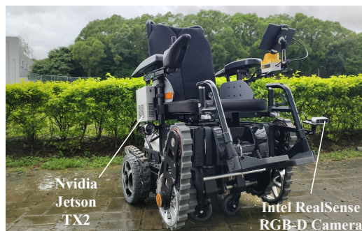
Fig. 1: The robotic wheelchair used in this work. It is equipped with an Intel RealSense RGB-D camera to collect data and an NVIDIA Jetson TX2 to run our S2P2 model.
