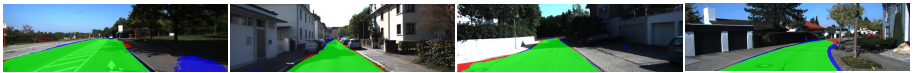
Fig. 8. Unsatisfactory results obtained using the KITTI road dataset. The true positive, false negative and false positive pixels are shown in green, red and blue, respectively (Color figure online).
