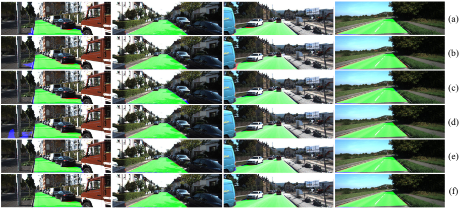
Fig. 7. Examples on the KITTI road benchmark, where rows (a)–(f) show the freespace detection results obtained by RBNet [10], TVFNet [17], LC-CRF [16], LidCamNet [5], RBNet [28] and our proposed SNE-RoadSeg, respectively. The true positive, false negative and false positive pixels are shown in green, red and blue, respectively (Color figure online).
